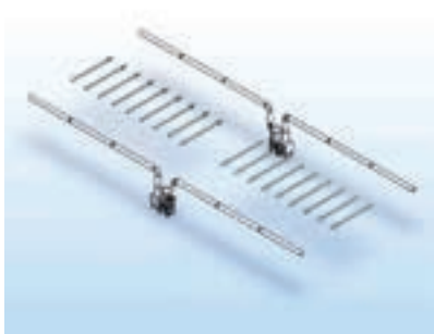
Double-parallel push/pull-system with 2 filter units and fans.
